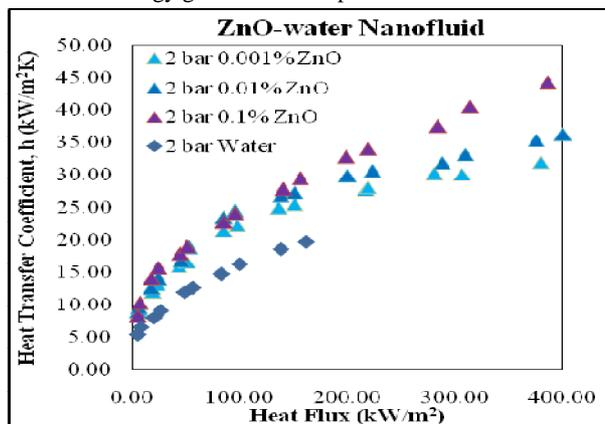
**Figure 4:** Variation of heat transfer coefficient with heat flux
