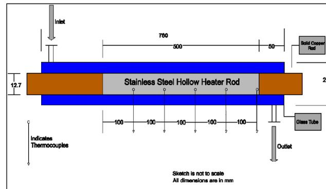
Figure 2: Test section and position of thermocouples
