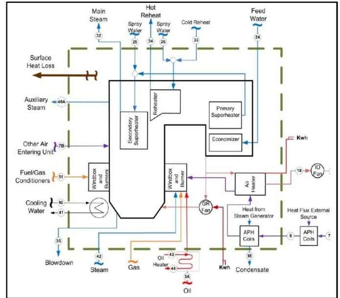
Figure 1: Steam boiler control volume according to PTC 4 standard [8].
