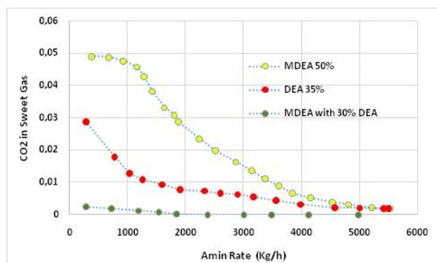
Figure 7: CO<sub>2</sub> content variation with different Amine solutions
