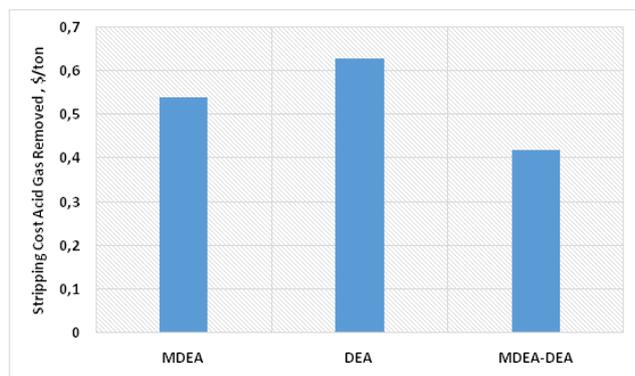
Figure 10: Economic Efficiency on Acid gas stripping
