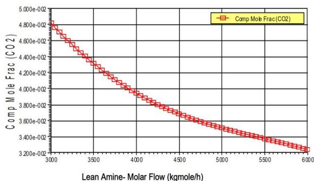
Figure 6: CO<sub>2</sub> content variation with Amine mas flow
