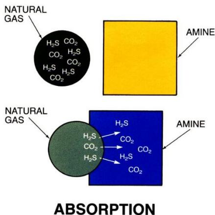
Figure 1: Amine chemical absorption
