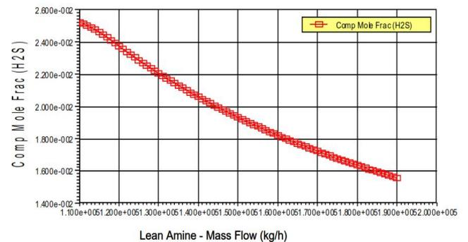
**Figure 5:** H<sub>2</sub>S content variation with Amine mass flow
