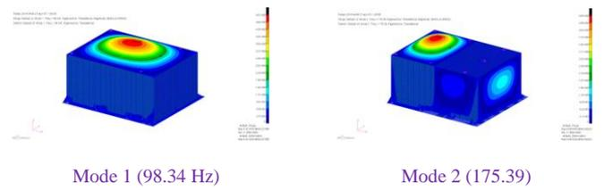
Figure 6: Mode shapes of Electronic Package using AL6061 material
