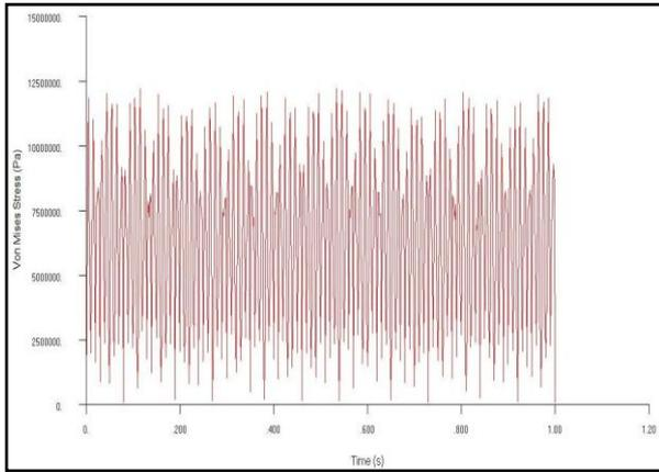
Figure 10: Stress-Time History for package made up of AZ31B
