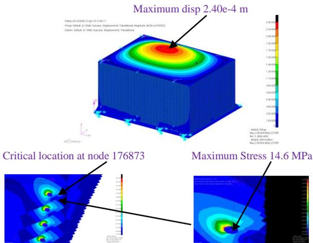
Figure 5: Displacement and critical location of Electronic package using AM162 material
