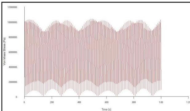
Figure 12: Stress-Time History for package made up of AM162
