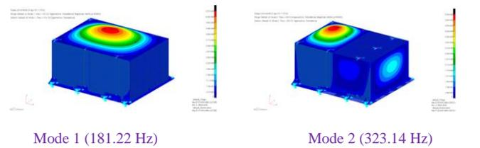
Figure 8: Mode shapes of Electronic Package using AZ31B material
