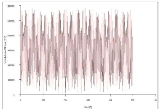
Figure 8: Stress-Time History for package made up of Al 6061
