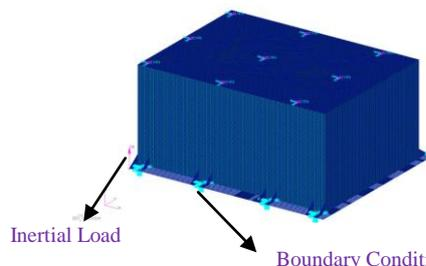
**Figure 2:** Boundary Conditions and Inertial load applied to the Package
