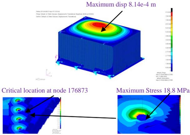
Figure 3: Displacement and critical location of Electronic package using AL6061 material
