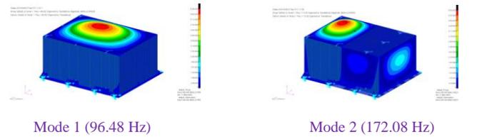
Figure 7: Mode shapes of Electronic Package using AZ31B material
