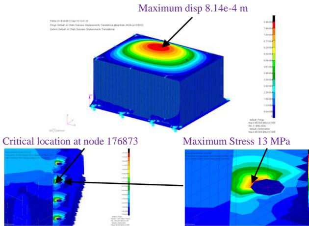
Figure 4: Displacement and critical location of Electronic package using AZ31B material
