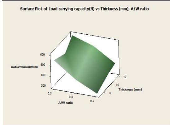
**Figure 5:** Surface plot of load carrying capacity v/s A/ W ratio and width.
