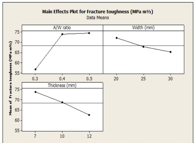
**Figure 4:** Main effect graph for mean Fracture toughness v/s A/W ratio, Width and Thickness.
