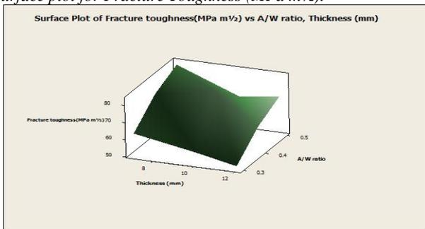
**Figure 7:** Surface plot for Fracture Toughness (MPa m<sup>1/2</sup>) v/s Thickness and A/W ratio.
