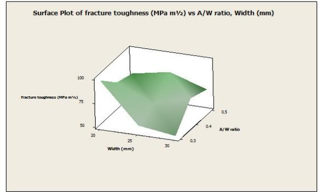
**Figure 8:** Surface plot for Fracture Toughness (MPa m<sup>1/2</sup>) v/s Width and A/W ratio.
