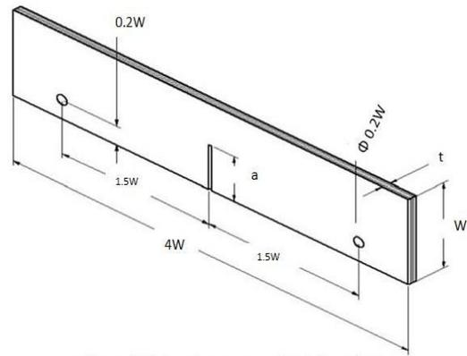
**Figure 1:** ENT specimen as per ASTM standard
