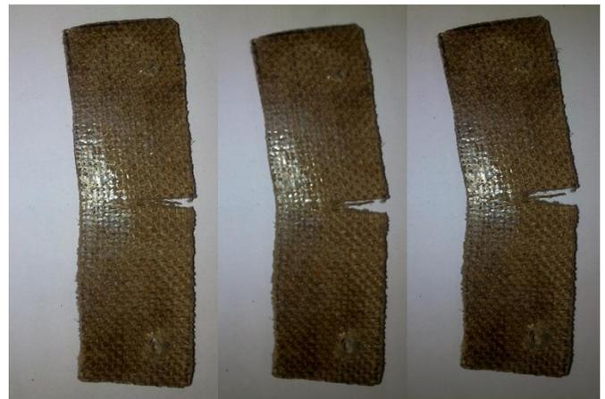
**Figure 2:** Fractured surface of specimens under ENT testing
