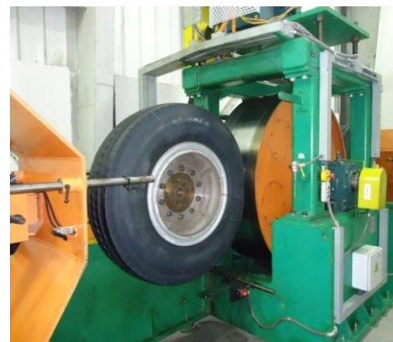
Figure 1: Indoor testing rig for bead durability
