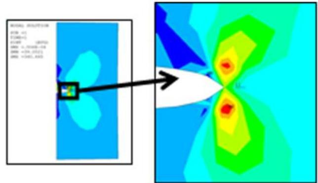
Figure 5: Stress concentration at crack tip
