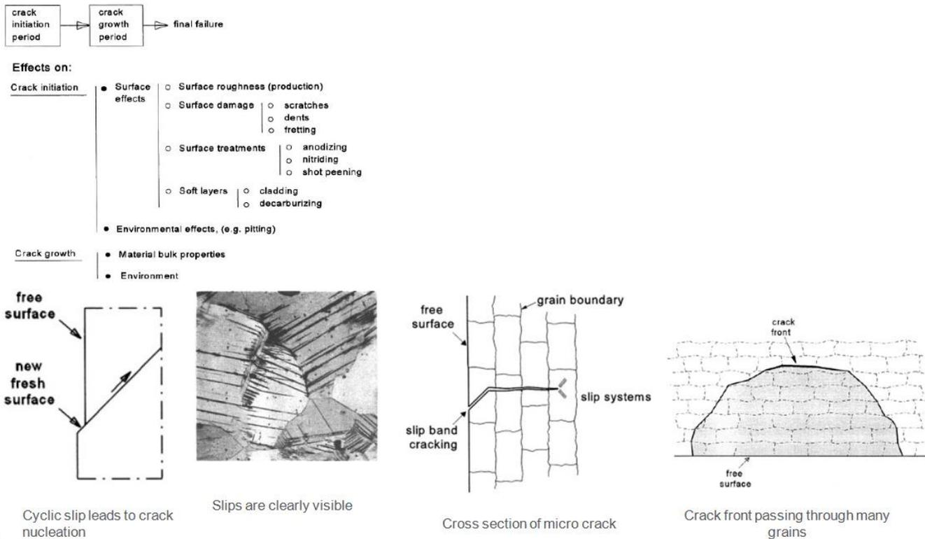
**Figure 2:** Crack growth mechanism flow to failure in metals
