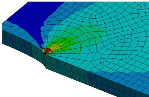
Figure 4: Stress concentration at crack tip
