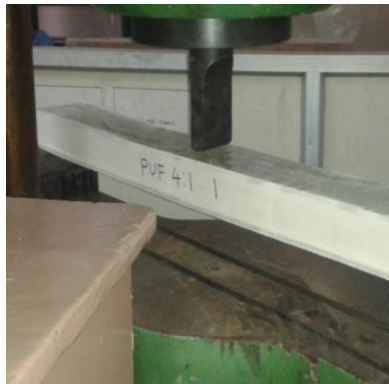
Figure 6: Flexure test of PUF 125-50mm thick
