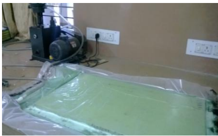
Figure 1: PUF 125 - 4:1-50mm, Vacuum bagging technique for fabrication of sandwich composites
