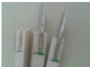
Figure 2: Tensile Test Specimens with GFRP attachments to be held at grips
