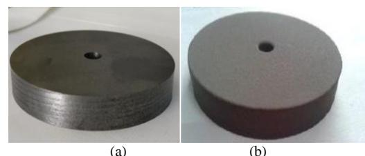
**Figure 1:** Uncoated (a) and coated (b) material of HVOF coating.
