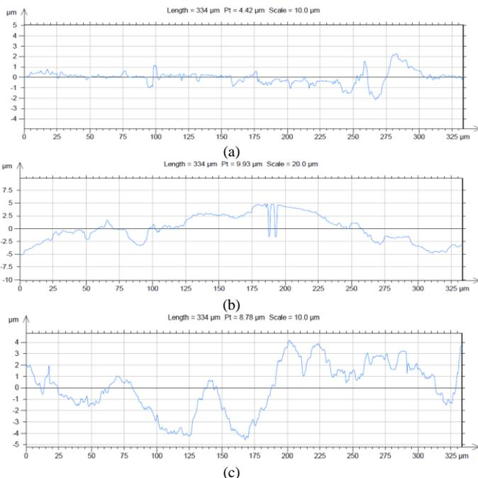
**Figure 5:** Surface roughness value patterns (a) Uncoated; (b) (80% Cr<sub>3</sub>C<sub>2</sub>+20% NiCr) Coated; (c) (75% Cr<sub>3</sub>C<sub>2</sub>+25% NiCr) Coated Material
