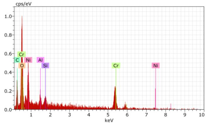
**Figure 3:** EDX analysis of the HVOF coating on (80%Cr<sub>3</sub>C<sub>2</sub>+20%NiCr).
