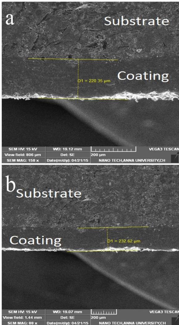
**Figure 2:** SEM image of HVOF coating (a) 80%Cr<sub>3</sub>C<sub>2</sub>+20%NiCr; (b) 75%Cr<sub>3</sub>C<sub>2</sub>+25%NiCr (Magnification - 200X)
