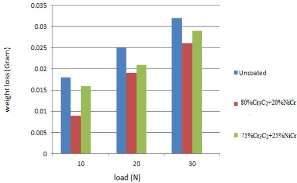
**Figure 7:** Comparison of weight loss due wear for the coated uncoated material for adhesive wear
