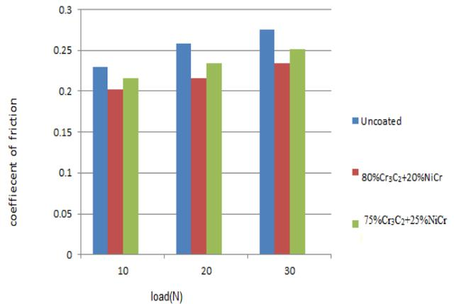
**Figure 6:** Coefficient of friction versus uncoated/coated material for adhesive wear
