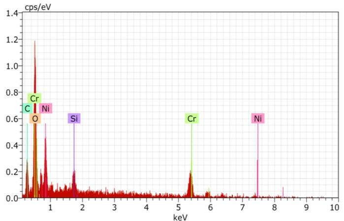
**Figure 4:** EDX analysis of the HVOF coating on (75%Cr<sub>3</sub>C<sub>2</sub>+25%NiCr).
