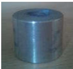
Figure 3: Compression test specimen
