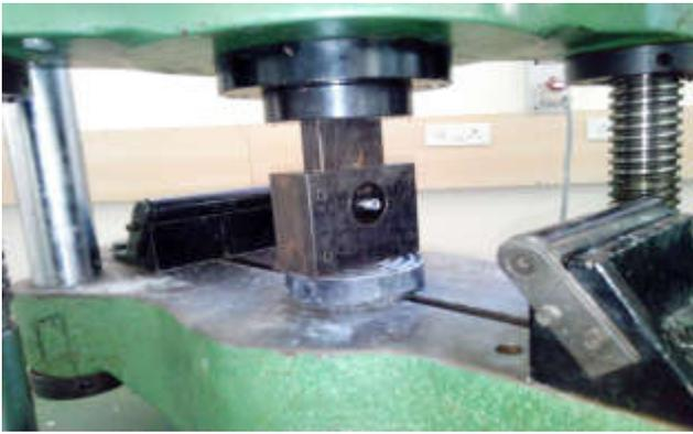
Figure 6: Shear test on UTM
