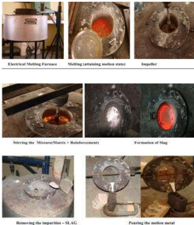
Figure 2: Steps in stir casting
