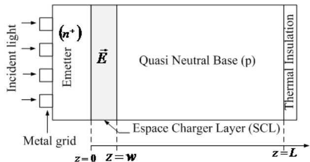
**Figure 1:** Schematic diagram of thermal insulation. The space charge layer (SCL) extends from  $z = 0$  to  $z = w$ . The quasi-neutral base extends from  $z = w$  to  $z = L$ .
