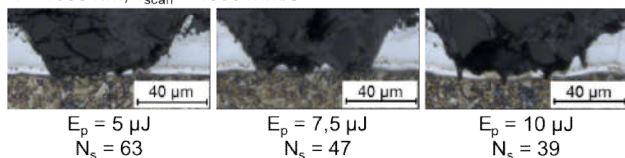
Figure 8: Removal depth as function of the number of scan N_s at v_{\text{scan}} = 1 \text{ m/s} and different pulse energies and for 515 \text{ nm} (above) and 1030 \text{ nm} (below)
