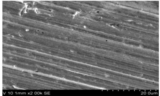
Figure 4: Wear groove of Fe based alloy coating [28]
