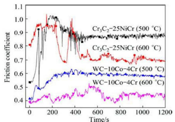
Figure 5: Coefficient of friction profile of Cr<sub>3</sub>C<sub>2</sub>-NiCr coating at elevated temperatures [59]
