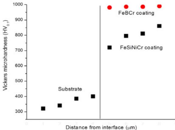
Figure 3: Microhardness profile of FeSiNiCr based alloy coating along cross section [29]
