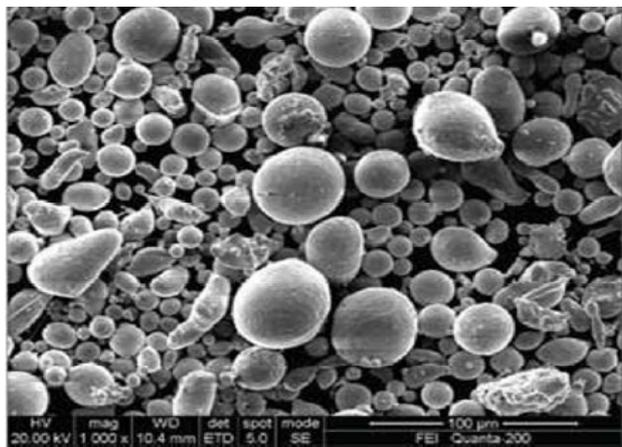
Figure 1: Cr<sub>3</sub>C<sub>2</sub>-NiCr powder image by SEM [59]
