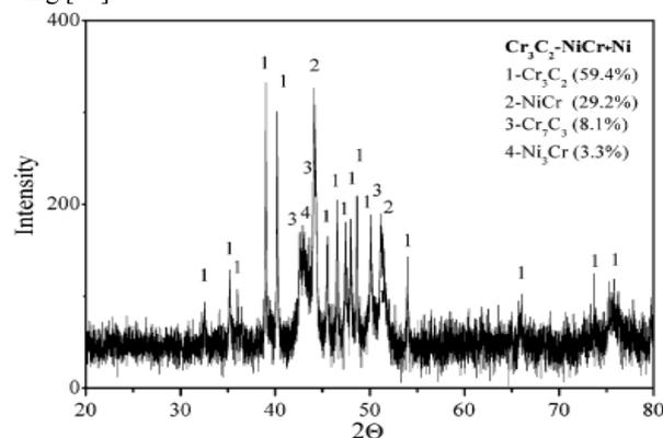
Figure 7: XRD analysis of Cr<sub>3</sub>C<sub>2</sub>-NiCr powder coating [60]
