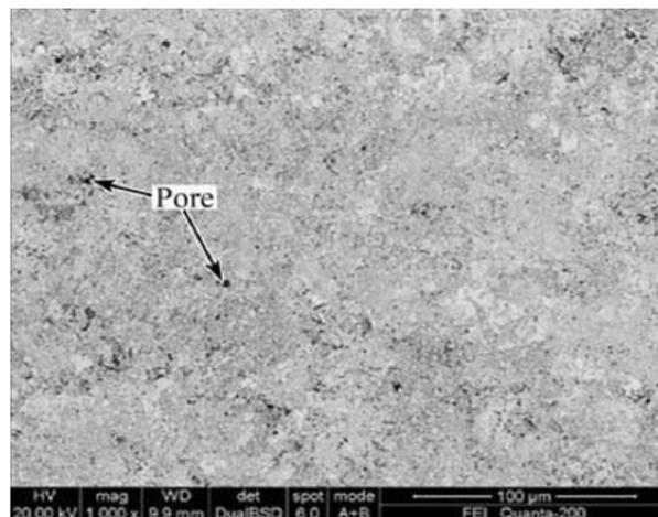
Figure 2: Porosity measurement by using SEM [59]
