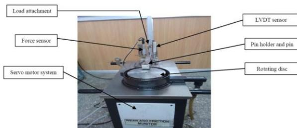
Figure 2: Actual Experimental Setup
