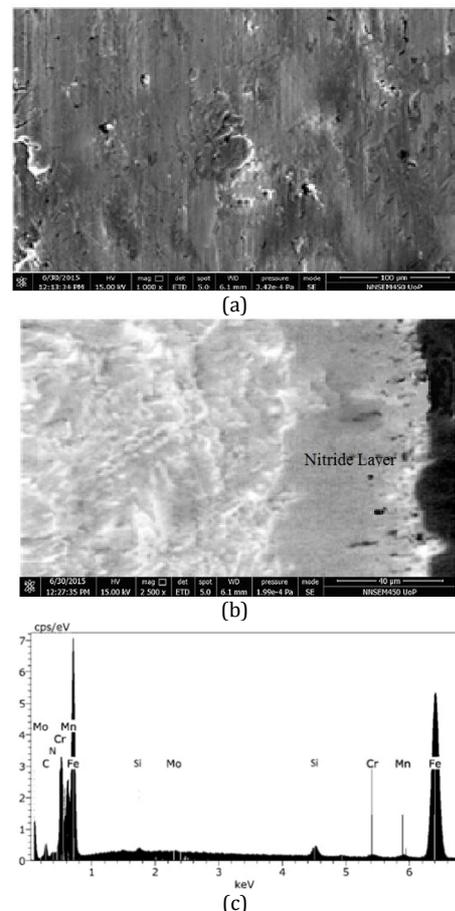
Figure 3: SEM micrograph of (a) cross-section of AISI 4140, (b) cross-section of nitrided 4140 and (c) EDX Spectrum of cross-section of nitrided 4140
