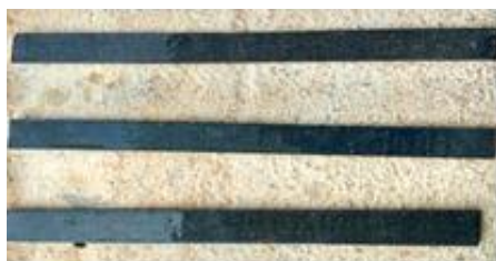
Figure 3: Fabricated specimens for tensile test as ASTM Standards
