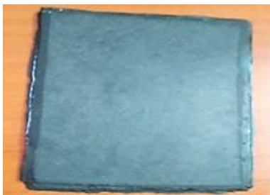
Figure 2: Fabricated Flax/Sisal/SiC nano powder/epoxy reinforced hybrid composite using hand layup process
