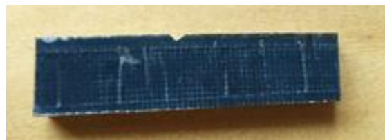
Figure 5: Specimen for impact test as ASTM standards
