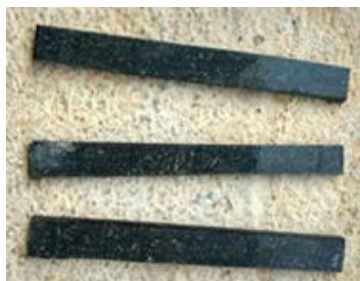
Figure 4: Specimens for flexural test as ASTM standards
