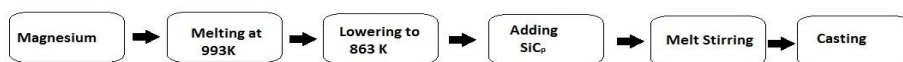
Figure 1: Fabrication of magnesium matrix composites reinforced with submicron \text{SiC}_p with the help of stir casting [10, 1]
