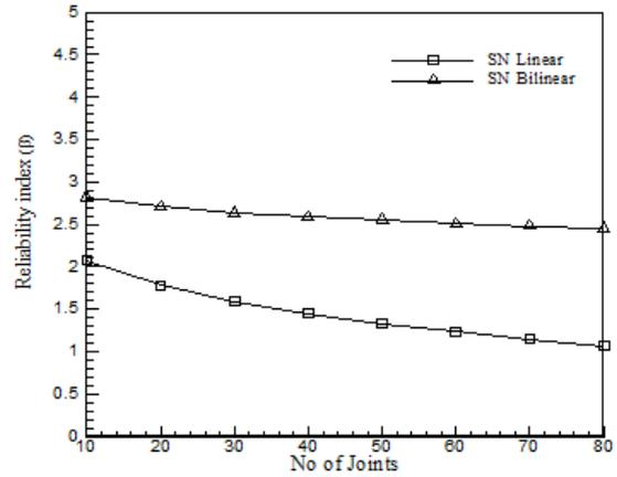
Figure 3: Comparison of reliability levels against variations in number of joints
