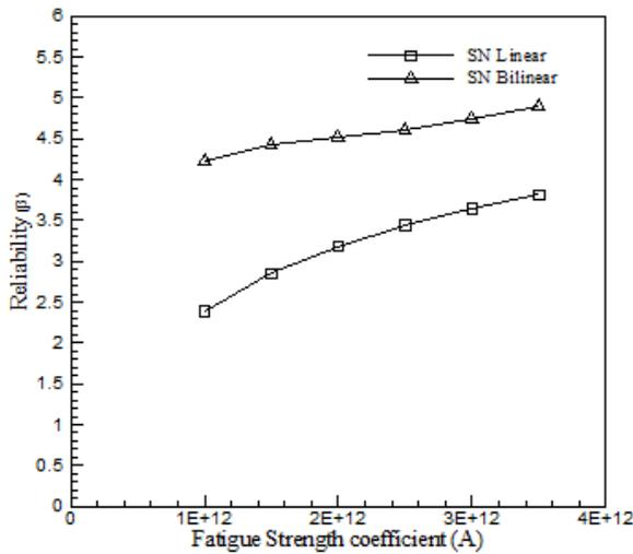
Figure 6: Comparison of reliability levels against fatigue strength coefficient (A)
