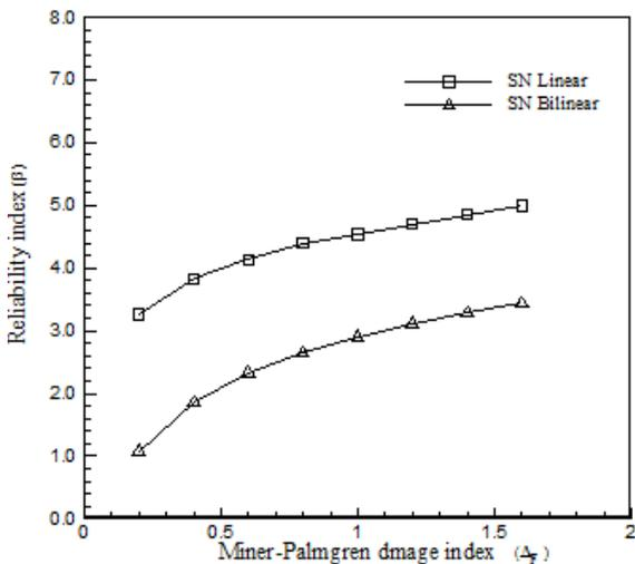
Figure 7: Comparison of reliability levels against variations in Miner Palmgren index
