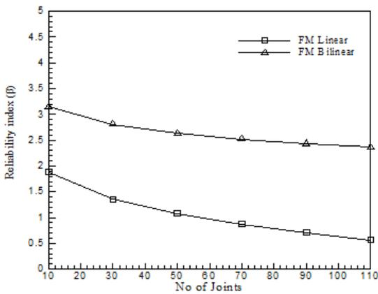
Figure 2: Comparison of reliability levels against variations in number of joints
