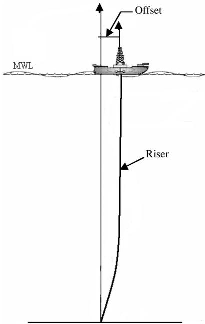
Figure 1: Typical Marine Riser
