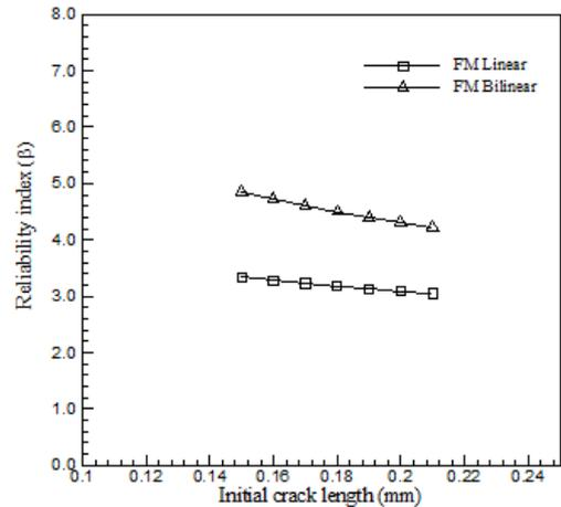
Figure 4: Comparison of reliability levels against variations in initial crack length (mm)
