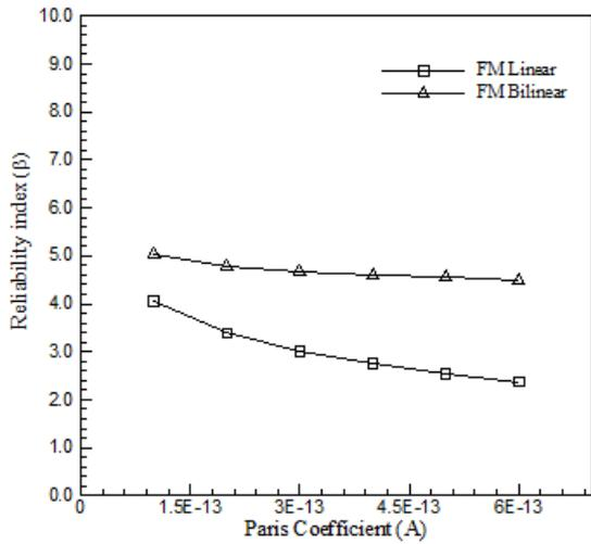
Figure 5: Comparison of reliability levels against variations in Paris coefficient (A)
