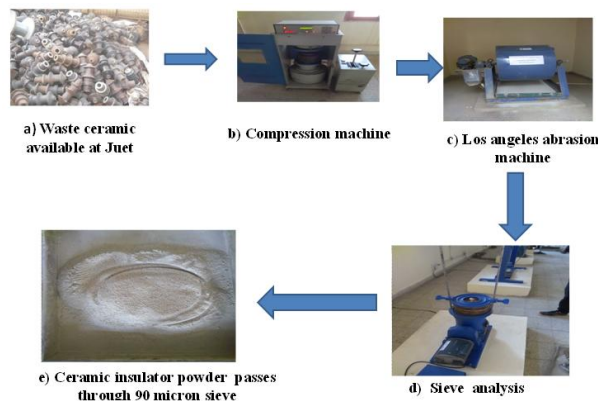
Figure 2: Processing of ceramic waste insulator [13]
