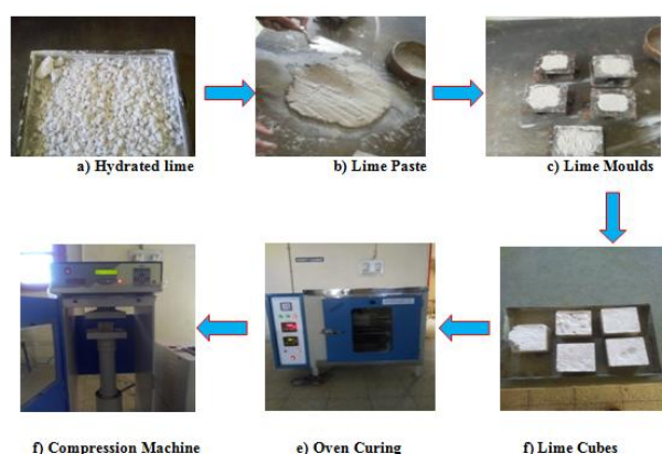
Figure 3: Lime reactivity test on ceramic waste insulator powder [13]
