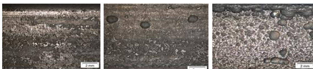
Figure 5: Corrosion on surface evolution from 30 to 90 days for H 2 S at 0.2mbar
