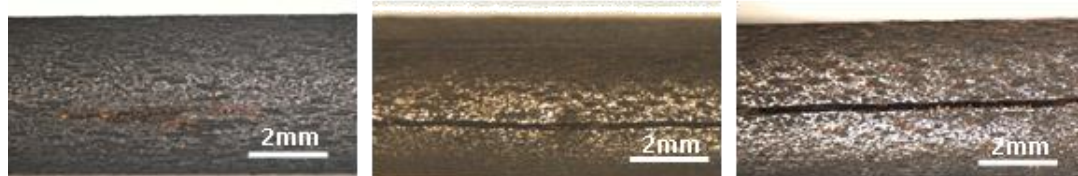
Figure 7: Hydrogen induced cracking growth vs test duration from 30 to 90 days for H 2 S content at 8mbars
