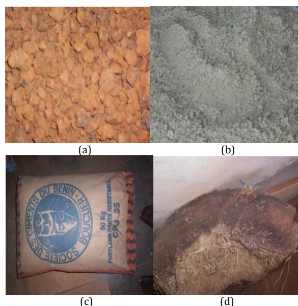
Figure 1: (a) Lateritic nodules from Avlamè quarry in Zogbodomey, (b) Lagoon sand of Dèkounbé, (c) cement CPJ 35, (d) Cup of borassus wood
