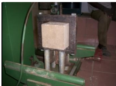
Figure 6: Conduct of the direct tensile test
