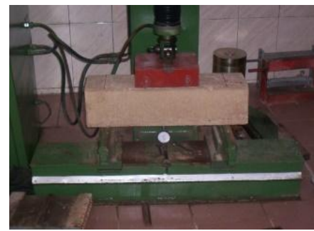
Figure 5: Execution of the 4-point bending test
