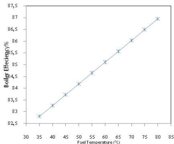
**Figure 2:** Effect of fuel temperature on boiler efficiency
