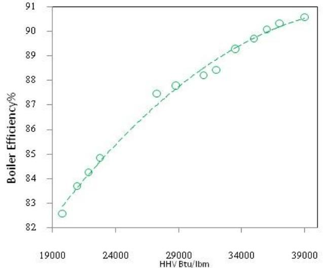
**Figure 6:** Effect of heating value of fuel on boiler efficiency
