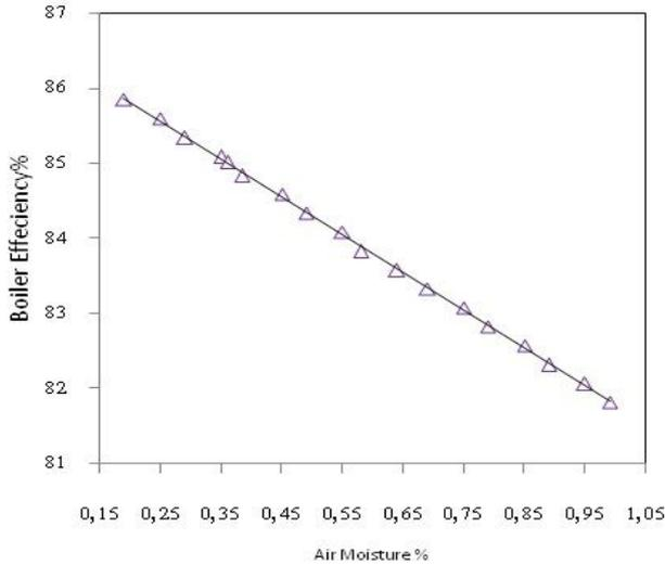
**Figure 4:** Effect of humidity on boiler's efficiency
