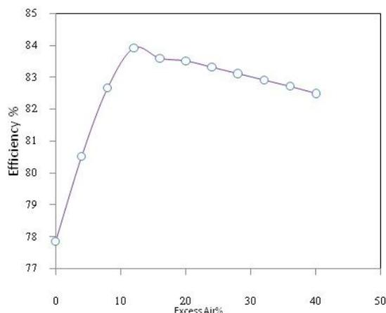
**Figure 3:** Impact of excess air on boiler efficiency
