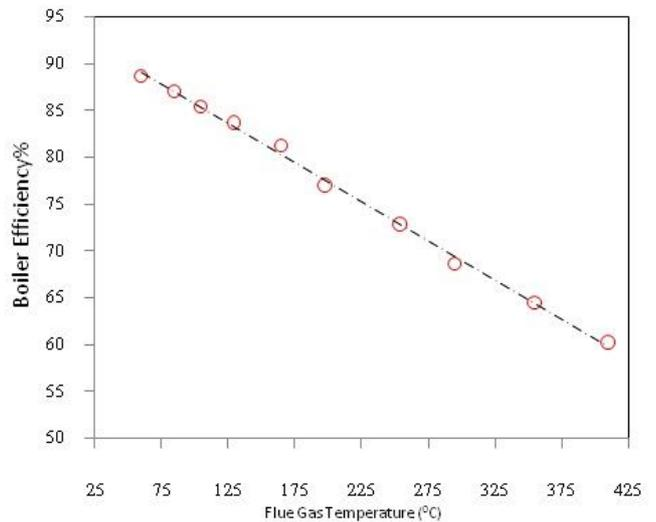
**Figure 7:** Effect of flue gas temperature drop on boiler efficiency
