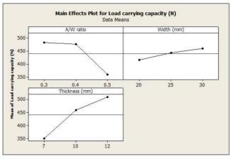
Figure 3: Main effect graph for mean load carrying capacity v/s A/W ratio. Width and Thickness.
