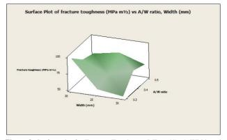
Figure 8: Surface plot for Fracture Toughness (MPa m½) v/s Width and A/W ratio.
