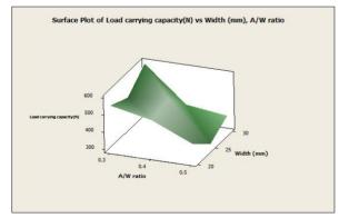
**Figure 6:** Surface plot of load carrying capacity v/s A/ W ratio and width. *Surface plot for Fracture Toughness (MPa m<sup>1</sup>/<sub>2</sub>):*
