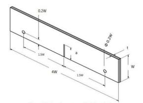
Figure 1: ENT specimen as per ASTM standard
