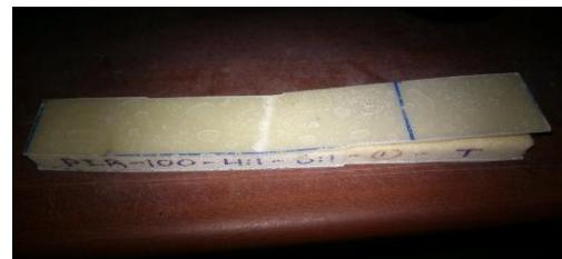
Figure 14: Laminate and core compression failure which leads to interface delamination
