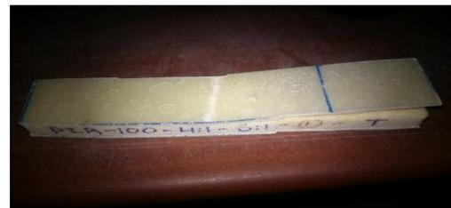
Figure 14: Laminate and core compression failure which leads to interface delamination
