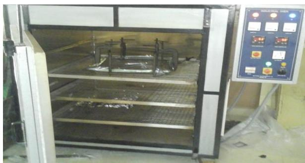
**Figure 2:** Platen compressed vacuum bag inside oven
