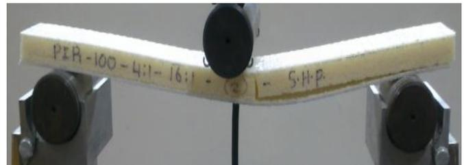
Figure 13: Core shear failure leading to interface failure
