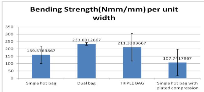
Figure 7: Type of technique Vs Bending strength per unit width
