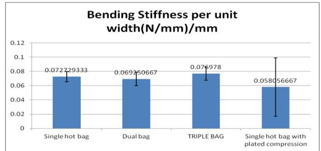
Figure 10: Type of technique Vs Bending Stiffness per unit width (N/mm)/mm
