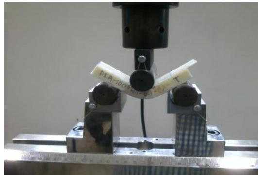
**Figure 5:** A specimen under 3 point bending with 6:1 span to depth ratio made by triple bag
