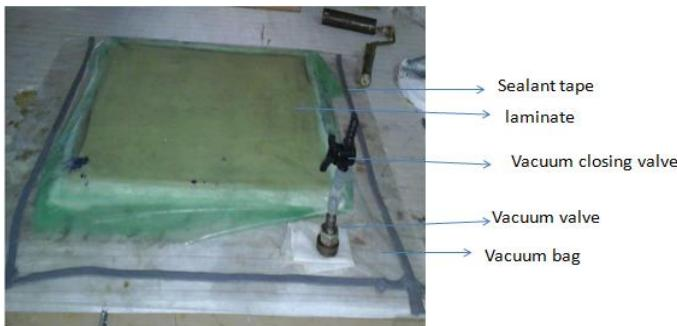
**Figure 1:** Sandwich panel inside the vacuum bag before high temperature curing
