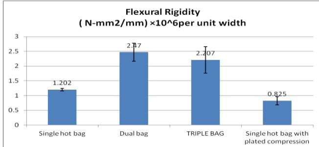
Figure 8: Type of technique Vs Flexural rigidity per unit width (N-mm<sup>2</sup>/mm) x 10<sup>6</sup>
