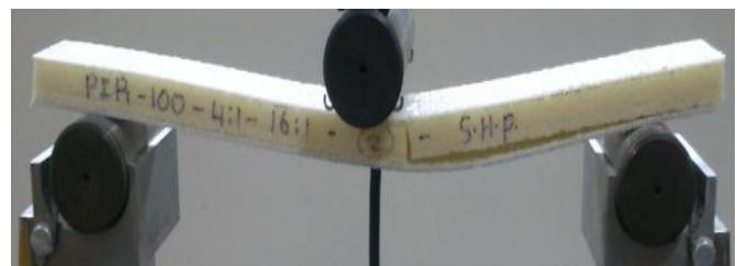
Figure 13: Core shear failure leading to interface failure
