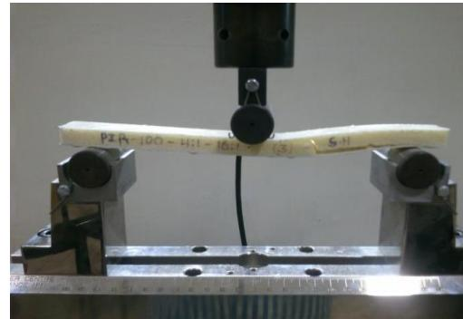
**Figure 3:** A specimen under 3 point bending with 16:1 span to depth ratio made by single hot bag
