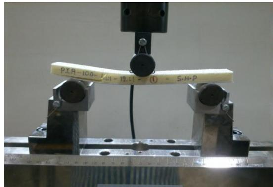
**Figure 6:** A specimen under 3 point bending with 12:1 Span to depth ratio made by plated compression
