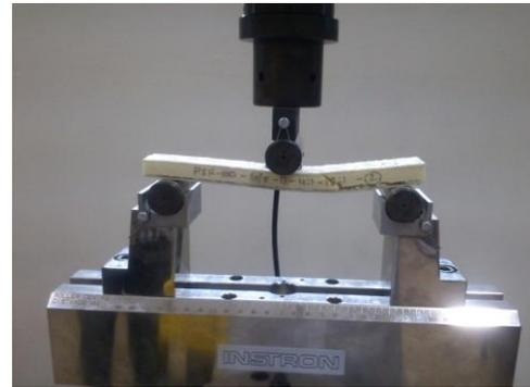
**Figure 4:** A specimen under 3 point bending with 12:1 span to depth ratio made by dual bag
