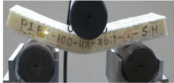
Figure 12: Core crushing failure leading to interface failure.
