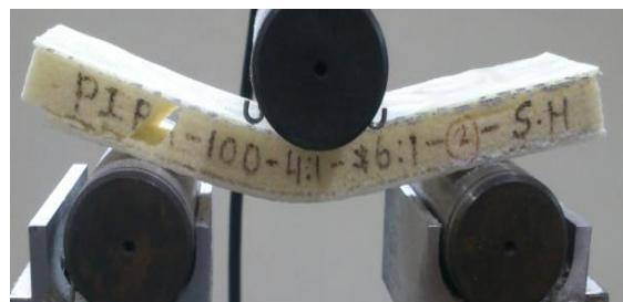
Figure 12: Core crushing failure leading to interface failure.
