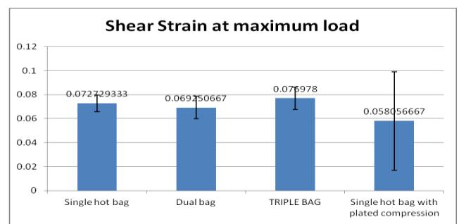
Figure 11: Type of technique Vs Shear strain at max load
