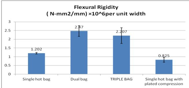
Figure 8: Type of technique Vs Flexural rigidity per unit width (N-mm<sup>2</sup>/mm) × 10<sup>6</sup>
