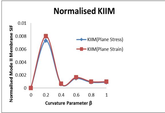
Figure 10 : Normalized Mode II Membrane SIF v/s Curvature Parameter  $\beta$
