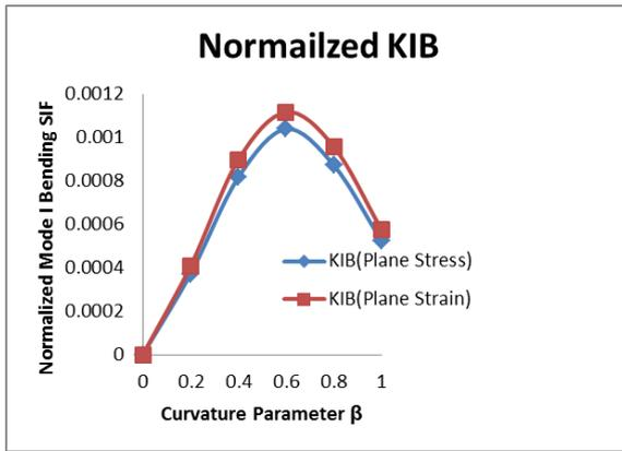
Figure 11: Normalized Mode I bending SIF v/s Curvature Parameter  $\beta$
