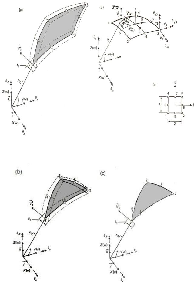
**Figure 1:** (a) Isoparametric quadrilateral shell element QUAD8; (b) Isoparametric triangular shell element TRIA6 and (c) singular Isoparametric triangular shell element STRIA6
