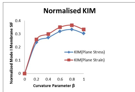
**Figure 9:** Normalized Mode I Membrane SIF v/s Curvature Parameter  $\beta$
