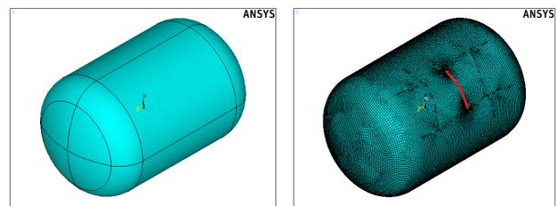
**Figure 6:** a) Geometric Model of cylinder with tori-spherical end closures b) FE Model of Circumferential Crack in cylindrical region
