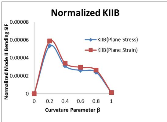
Figure 12: Normalized Mode II Bending SIF v/s Curvature Parameter  $\beta$
