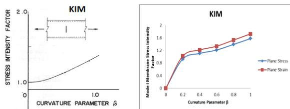
**Figure 4:** Mode I membrane SIF-Target solution and Present Analysis
