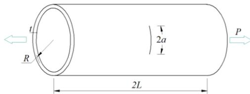
**Figure 3:** Axial loaded cylinder with a circumferential crack
