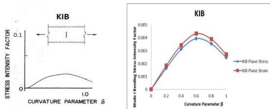
**Figure 5:** Mode I bending SIF-Target solution and Present Analysis
