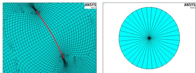
**Figure 7:** Circumferential crack **Figure 8:** Crack tip singular elements
