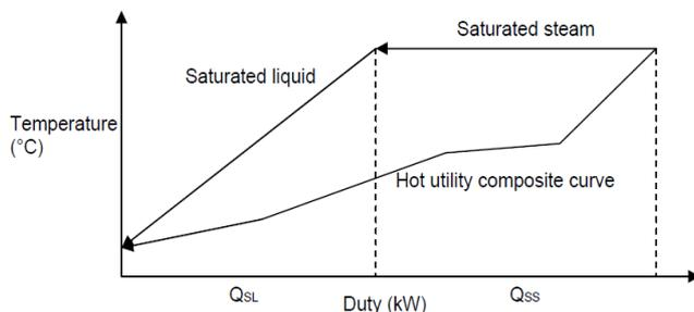
Figure1: targeting using saturated steam as well as saturated liquid.
