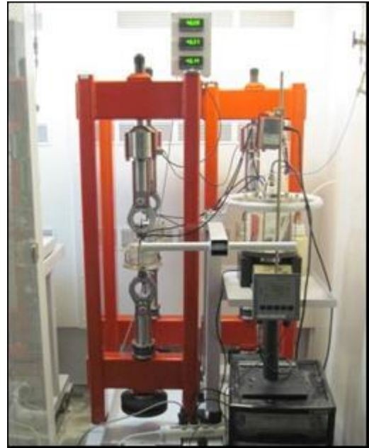
Figure 2: Sulphide Stress Cracking device to stress the sample up to 100kN with an uniaxial strength
