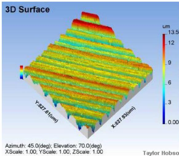
Figure 6: 3D Surface roughness for uncoated specimen
