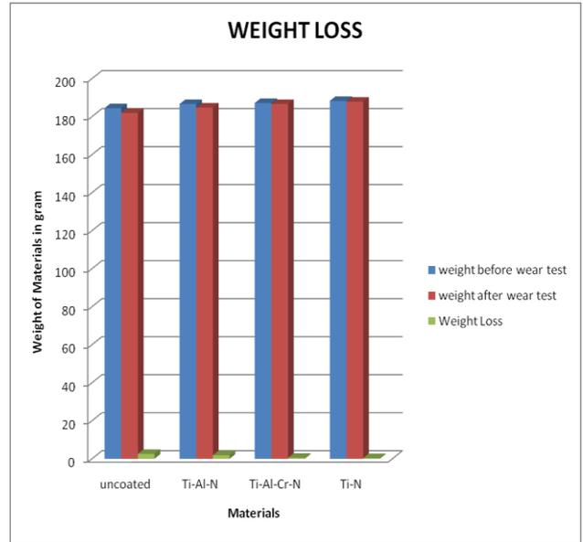
Figure 4: Weight loss chart at ambient conditions
