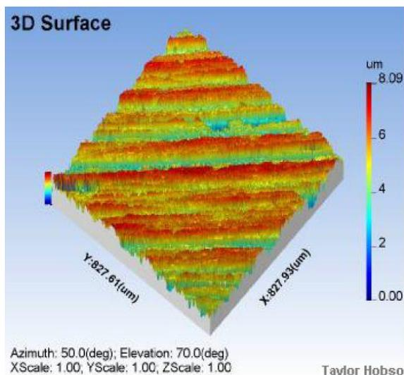
Figure 7: 3D Surface roughness for coated specimen
