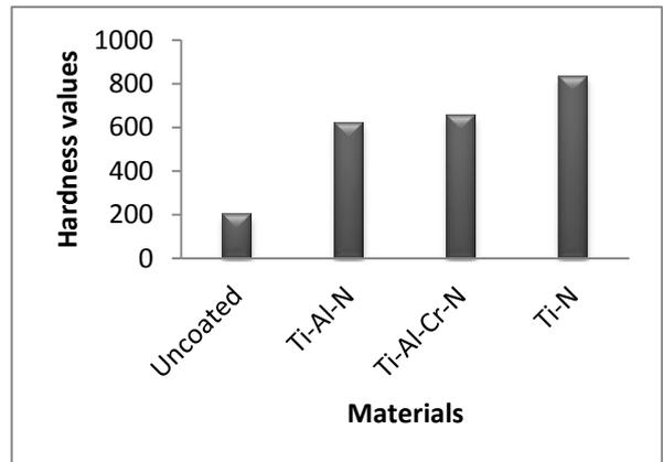
Figure 5: Microhardness graph plot between coated and uncoated materials
