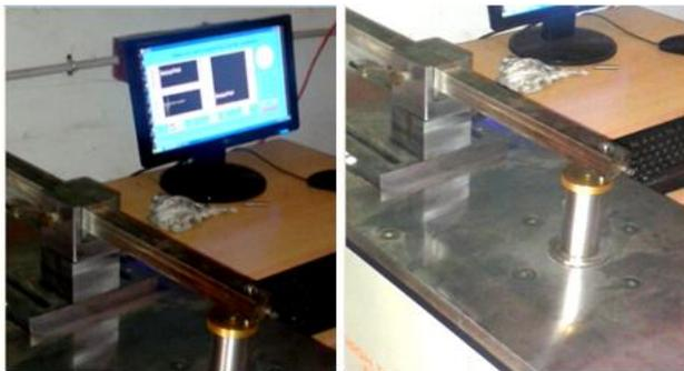
**Figure 1:** Experimental setup of Pin-On-Disc apparatus**Table 3:** Specification of pin-on-disc apparatus
