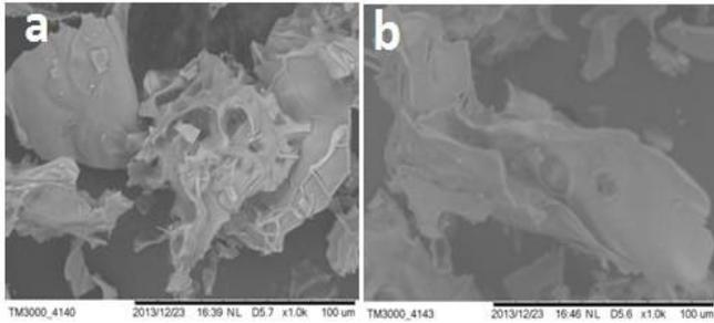
Figure 2: (a-b): SEM micrographs of  $\alpha$ -Al<sub>2</sub>O<sub>3</sub> nanoceramics
