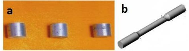
Figure 5: (a) specimen of compression strength and hardness test, (b) specimen of ultimate tensile strength tests
