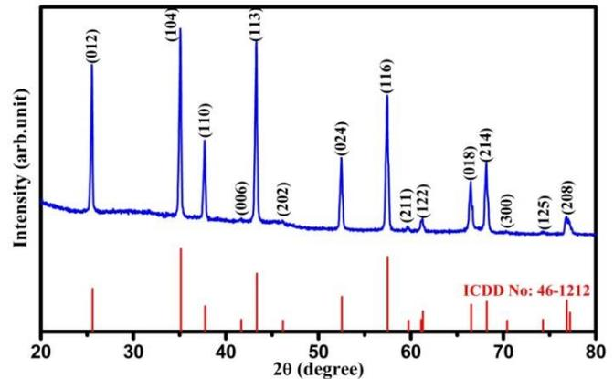
**Figure 1:** PXRD patterns of  $\alpha$ -Al<sub>2</sub>O<sub>3</sub> nanoceramics
