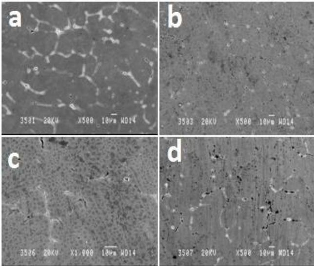
Figure 4: a) SEM micrograph of matrix, b) SEM micrograph of 2% MMCs, c) SEM micrograph of 4% MMCs and d) SEM micrograph of 6% MMCs)
