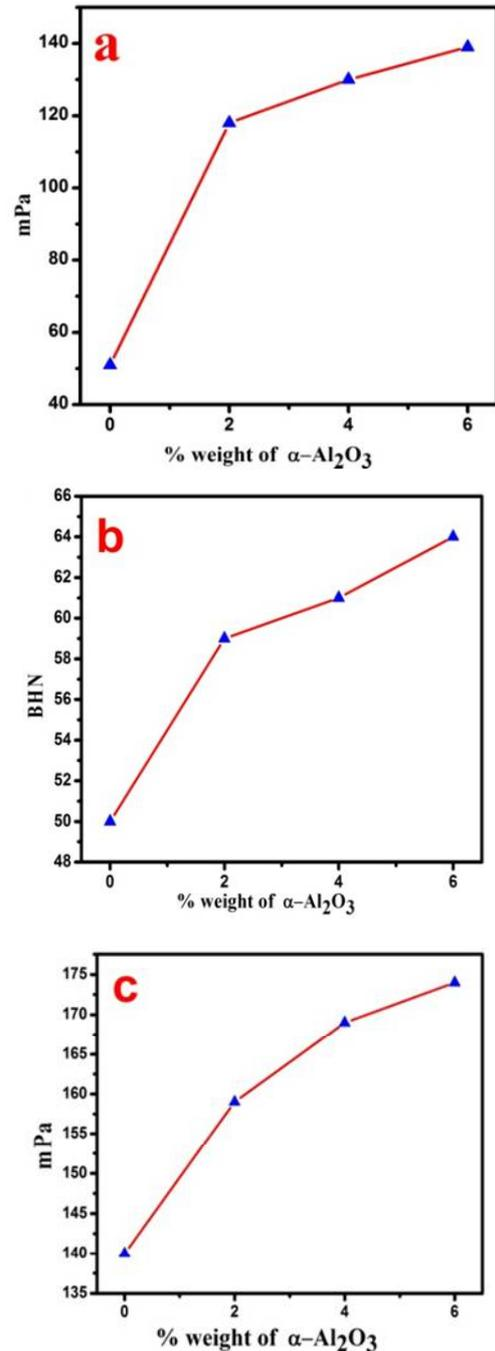
Figure 6: (a) Plot of ultimate tensile strength, (b) Plot of hardness, (c) Plot of compression strength
