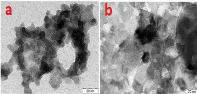
Figure 3: (a-b): TEM micrographs of  $\alpha$ -Al<sub>2</sub>O<sub>3</sub> nanoceramics at different magnifications
