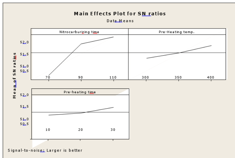
Figure 3: Main effects plot for s/n ratio for Impact strength
