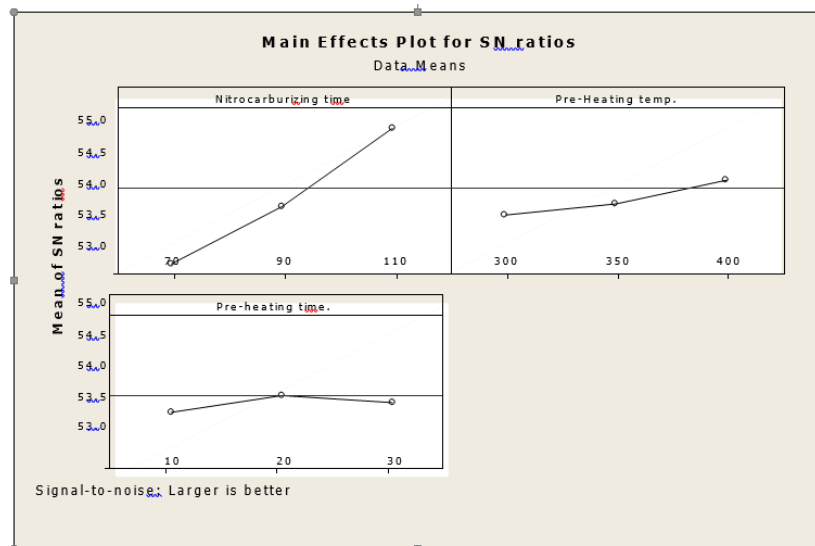
Figure1: Main effects plot for s/n ratio for Micro-hardness
