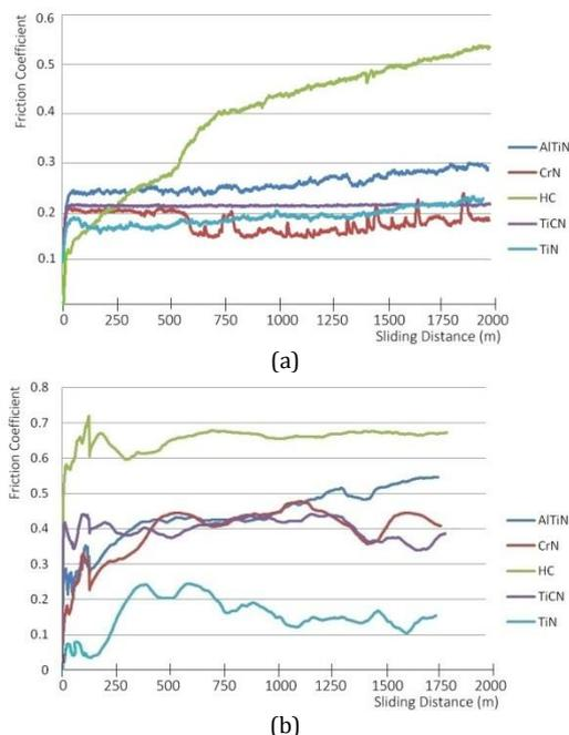
**Figure 5:** Variation of friction coefficient in dry sliding condition at (a) 10N and (b) 20N load
