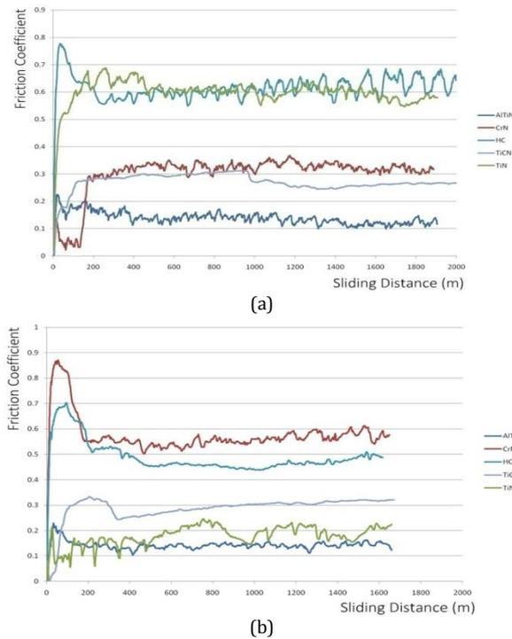
**Figure 7:** Variation of friction coefficient at 4.19 m/s in (a) dry and (b) wet sliding condition
