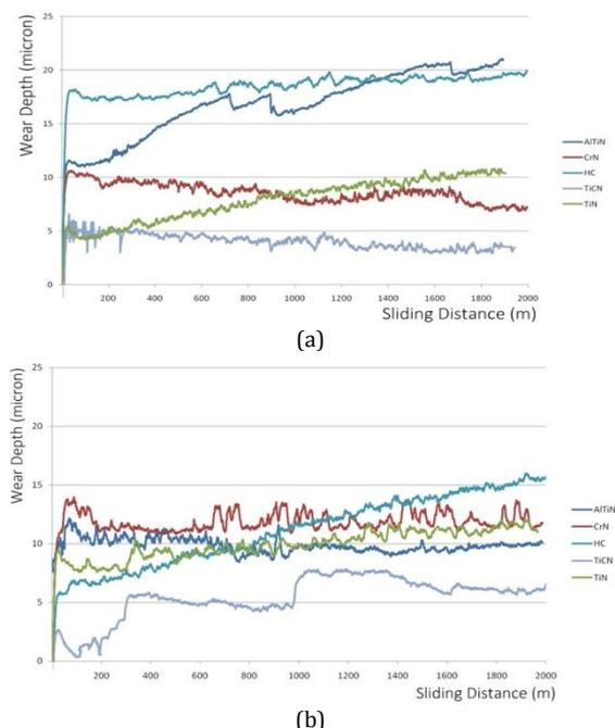
**Figure 6:** Variation of wear track depth in dry sliding condition at (a) 4.19 m/s and (b) 5.23 m/s
