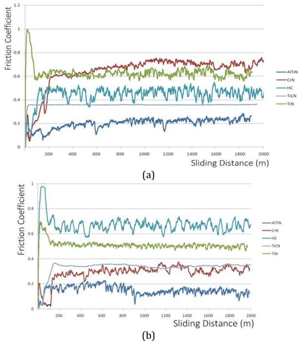
**Figure 8:** Variation of friction coefficient at 5.23 m/s in (a) dry and (b) wet sliding condition
