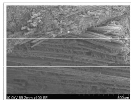
Figure 11: Fatigue failure of cross ply
