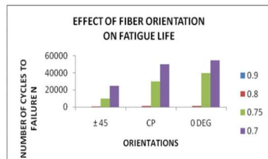
Figure 4: Orientation effect on life of Composites
