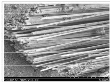
Figure 10: Broken bundles of uni-directional ply under fatigue loading
