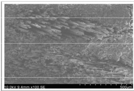
**Figure 13:** Fatigue failure of  $\pm 45$  degrees sample
