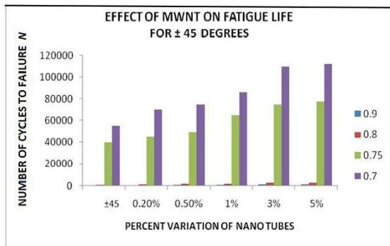
Figure 5: Effect of MWCNT on angle ply
