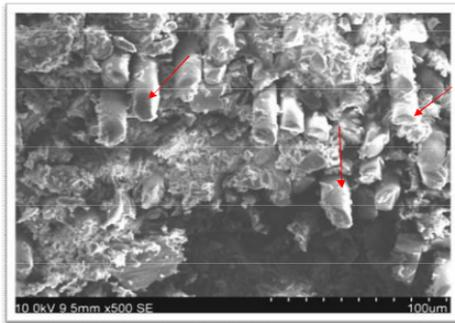
**Figure 12:** Dense network of broken fibre stubs indicated by arrows
