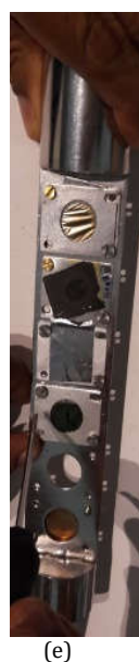
Figure 1: (a) Cr deposited copper foil sandwiched in between two stainless steel target frame (b) immersed in diluted \text{HNO}_3 (c) self-supporting thin film of chromium (d) iron and vanadium target (e) various targets placed in target ladder
