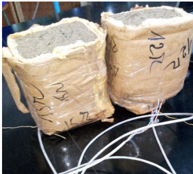
Figure 5: Samples embedded in glass wool with thermocouple and Peltier element underneath
