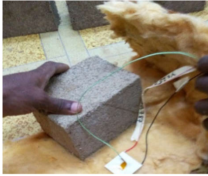
Figure 4: Peltier Element and Thermocouple Sensors Under a Sample
