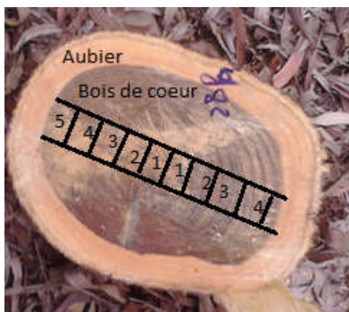
Figure 1: Picture showing the cutting of the samples and their numbering from pith to sapwood
