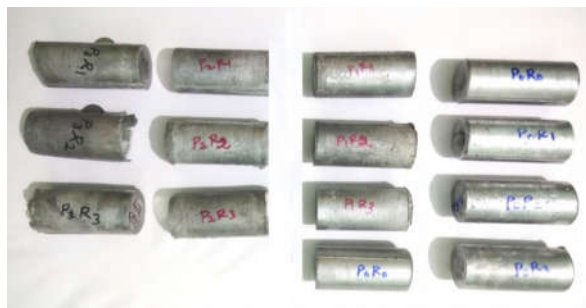
Figure 1: Specimens prepared by varying the weight % of reinforcement and Squeeze Pressure
