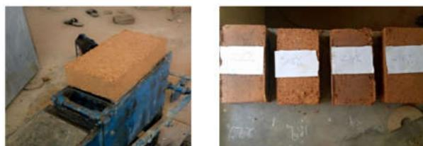
**Figure 7:** Making bricks with a press (left) and a cure (right)
