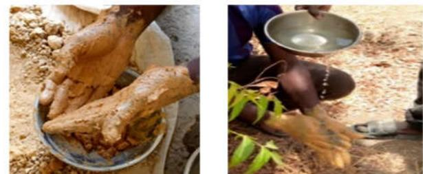
**Figure 4:** Hand Washing Test
