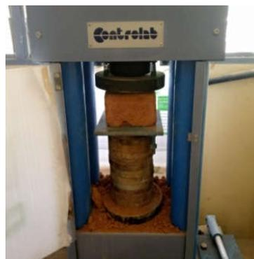
**Figure 8:** Crushing test of a compressed brick
