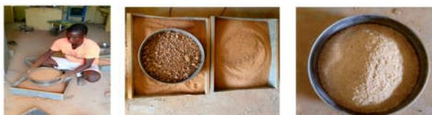
Figure 6: Soil sieve on 5 mm sieve (left and middle) and rice bran (right)
