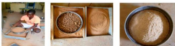
**Figure 6:** Soil sieve on 5 mm sieve (left and middle) and rice bran (right)
